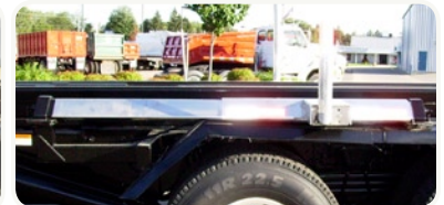
• Adjustable Sliding Pivot Fits Even Older Style Hoists And Adjusts Forward And Backward To Easily Accommodate Varying Length Containers From 10 To 50 Cubic Yards.
