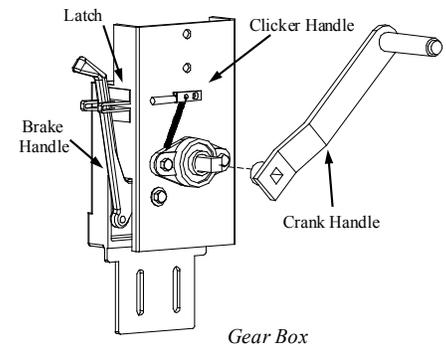
Warning: Do not release brake without **REMOVING THE CRANK HANDLE**. Do not release handle unless ratchet pawl is properly engaged. Do not disengage ratchet pawl unless tension is applied to handle. Failure to observe these warnings will cause handle to turn out of control and could cause personal injury.
